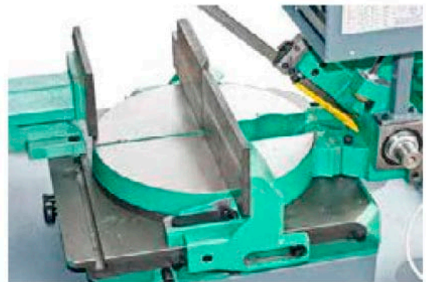
Large circular table rotating together with the bow to ensure optimal support of the piece to be cut
