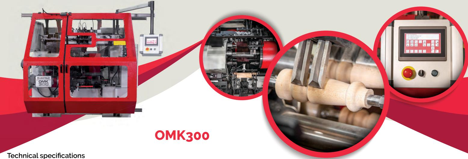
Automatic hydro-pneumatic multi-spindles machine for turning and sanding wooden pieces with a maximum length of 300mm and a maximum square of 100x100mm (on request, it's possible to machine a maximum square of 120x120mm).
