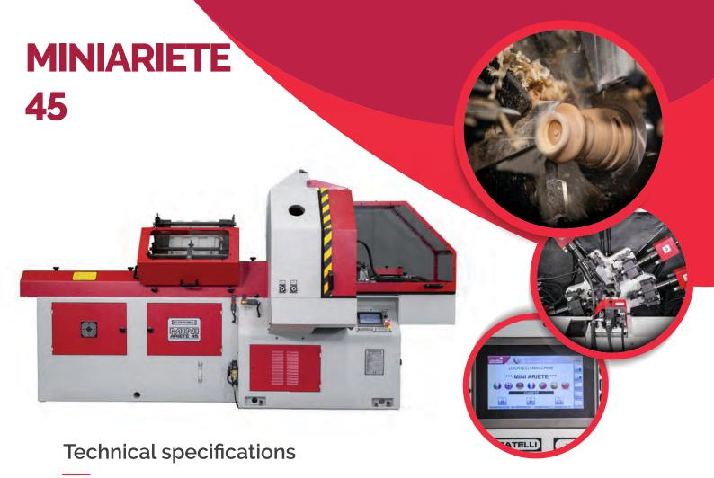
Fully automatic LOCATELLI lathe with PLC Control with touch screen for mass production of small turned wooden items till 45mm diameter like wooden toys, bottles capsules, knobs, handles and many others.
