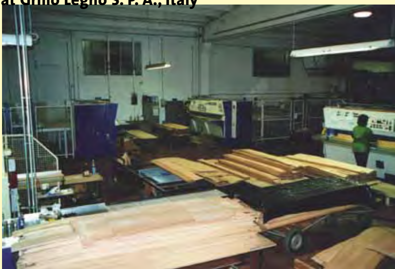
Crossfeed splicer at Grillo Legno S. P. A., Italy
