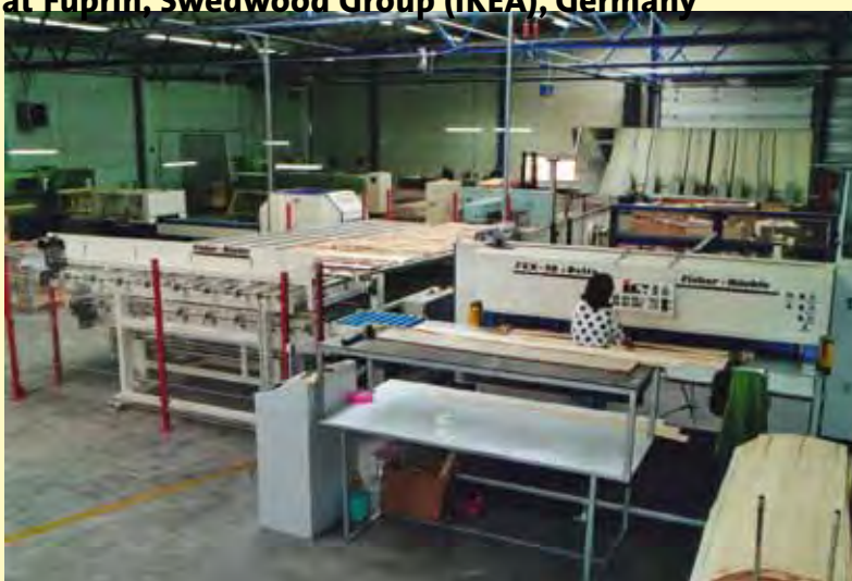
Crossfeed splicer at Fuprin, Swedwood Group (IKEA), Germany
