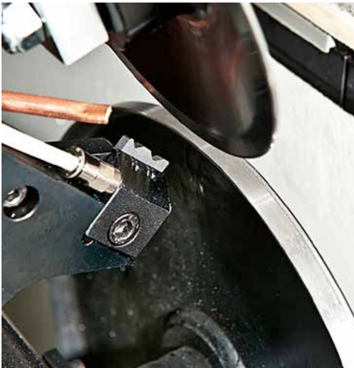
Version for automatic processing of 2 rounded edges by HMI. Micro-adjustments with NC axes (opt).
