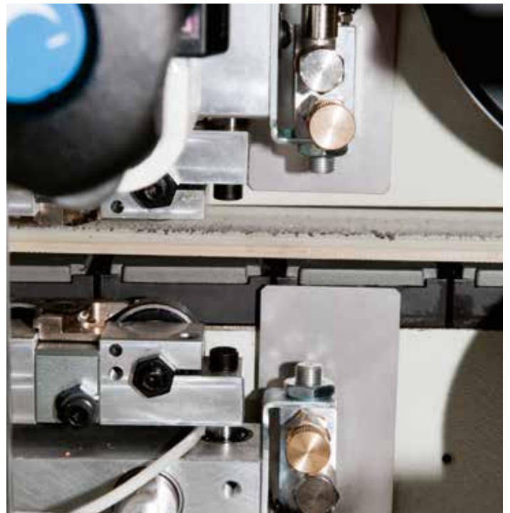
Liquid for smoothing the plastic edge and for brightening the ABS edge (opt.).
