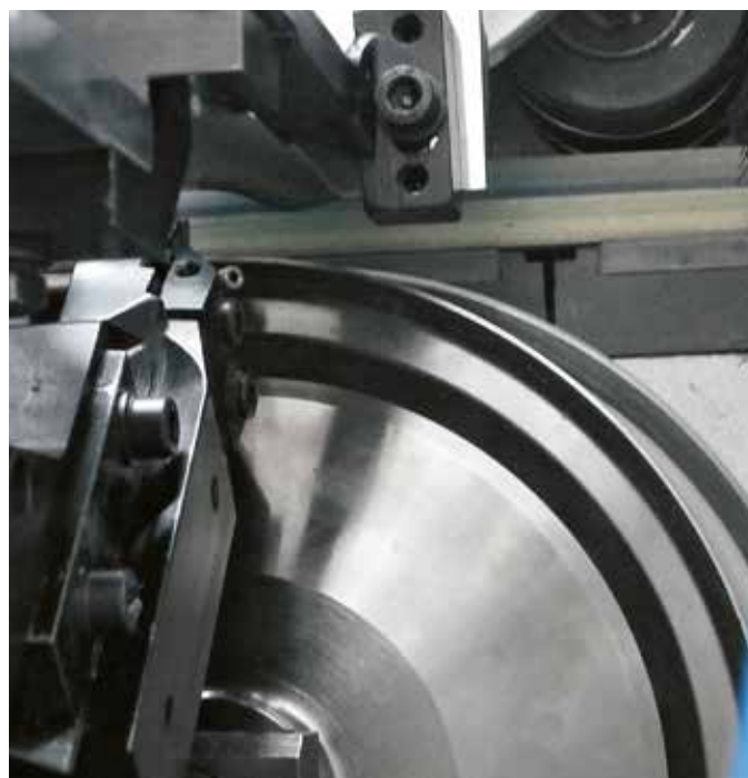
Twin Feeler copying system allowing a constant processing, without marks, especially at high speeds.
