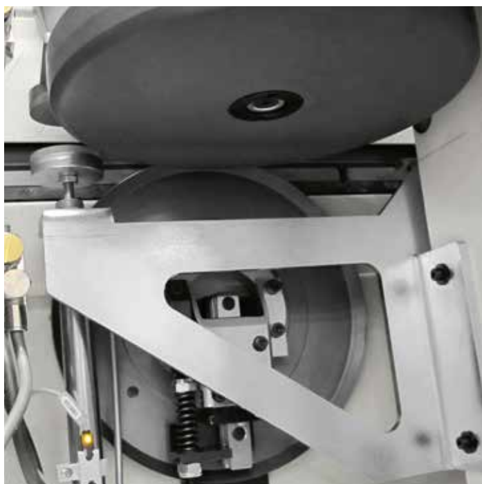
Additional opposite-copying system with large diameter disc. For processing of panels with reduced thickness and tendency to bend.
