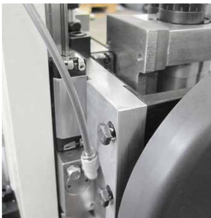
Nesting lock kit. It stops instantly the vertical copying movement in the presence of nesting holes (opt.).
