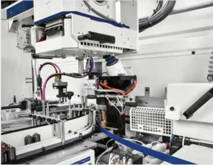
2 or 6 coil magazine (opt.) with possibility of adding one coil manually for occasional processing. Highly reliable system by rollers for the edge exchange.
