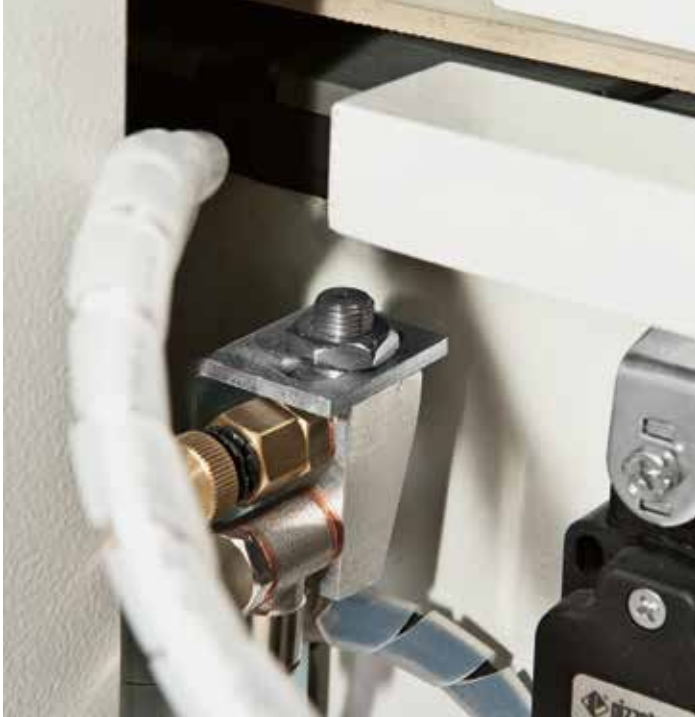
Anti-adhesive liquid to prevent the adhesion between panels due to the scraps of the glue when forming stacks of machined panels (opt.).
