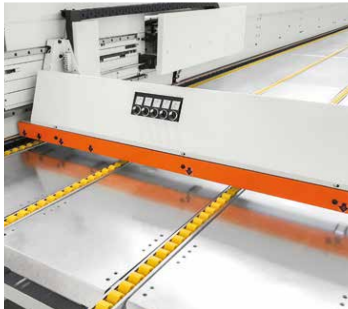
M+ manual infeed device for easy and error-free introduction of panels orthogonally to the feed direction. For dimensions up to 2600 mm (opt).
