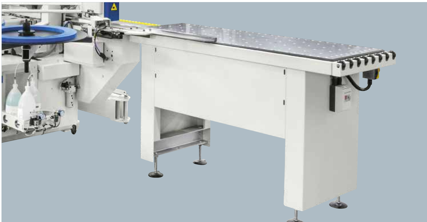
Easy and fast handling of panels in the loading area with the air cushion table (opt).
