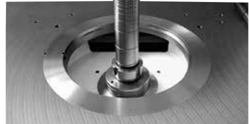
Interchangeable spindle with MK4 fitting on t 60f and MK5 on t 70f for using tools with different hole diameters thanks to the possibility of rapid changing of the spindle.
